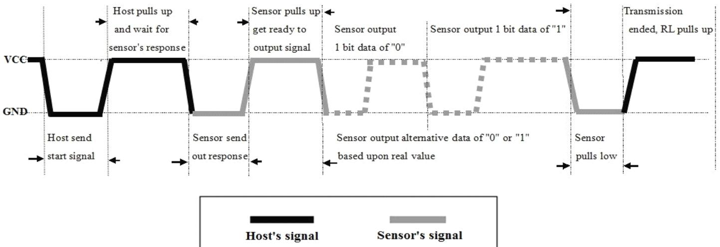
1) Step 1: MCU send out start signal to AM2302 and AM2302 send response signal to MCU
